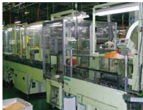
Lead-free high-temperature soldering equipment at the Fujiyama Works
